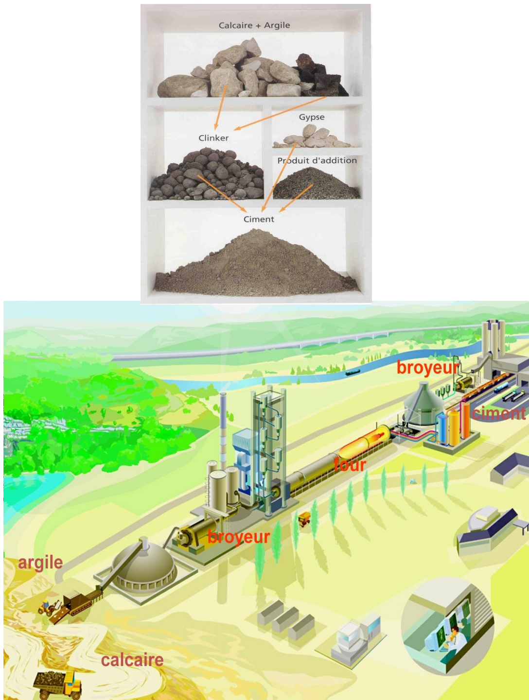
Figure I.1 Le four de fabrication de ciment [12].
